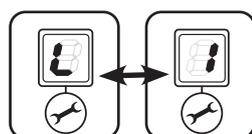
4. Once the displays shows "L" and "1" as shown in the previous picture, press the reset button until the display shows the letter "P" on the **boiler**
