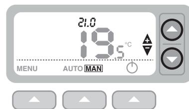
To test that the thermostat is paired and working, set the Thermostat to "MAN" and raise the temperature using the to maximum. If connected correctly after a few seconds the boiler will fire.
